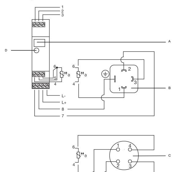
А Setup connection and connection for teach-in connector (on the JUMO ecoTRANS Lf 02)
